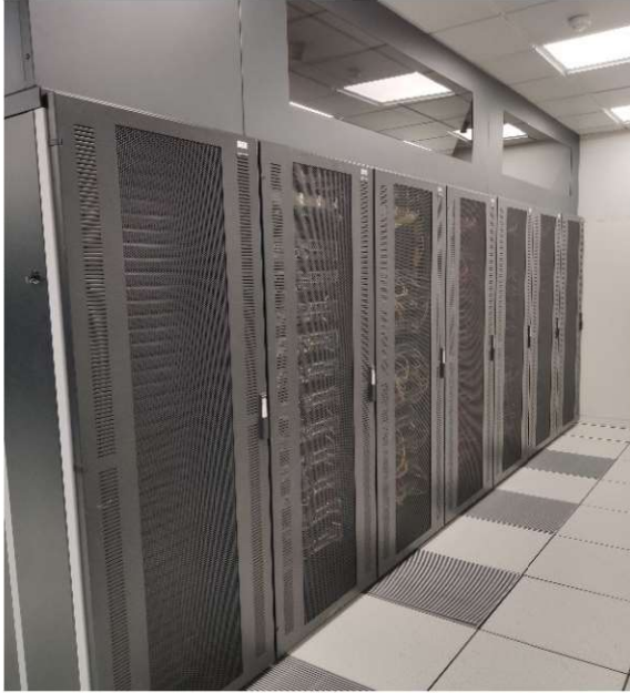
The bank HPC Cluster : 44,000 xeon cores – 450 kW - in only ten racks !
