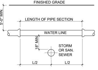
WATER & SEWER LINES PERPENDICULAR
